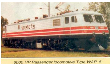
6000 HP Passenger locomotive Type WAP 5
